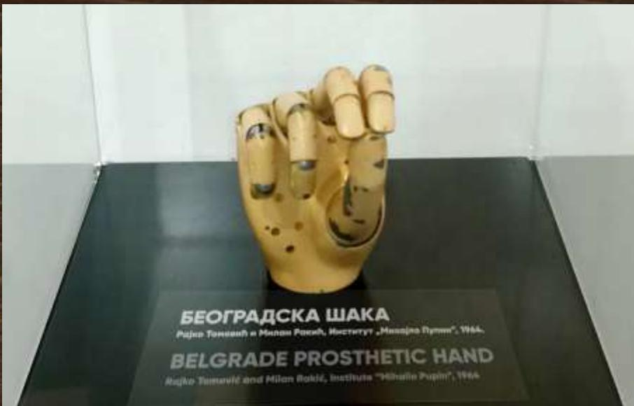
Belgrade fist as a terminal organ of "Minski Hand". This system was essential hardware for the development of artificial intelligence for robot control. The system included the Belgrade Hand as the only self-adjusting gripping object to be captured.
